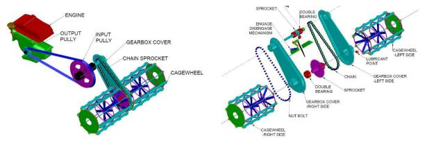
Fig. 7: Power transmission system of Hydro tiller.
